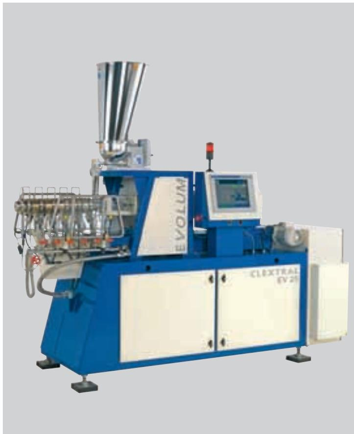
This machine, the smallest extruder in the EVOLUM range, offers the same technological advantages and performance as the other models in this series: high torque, and fast screw rotation for high output. It features a temperature control system which heats and cools each barrel module independently and a variable speed drive to regulate the screw speed. An automatic barrel opening system is an available option.
