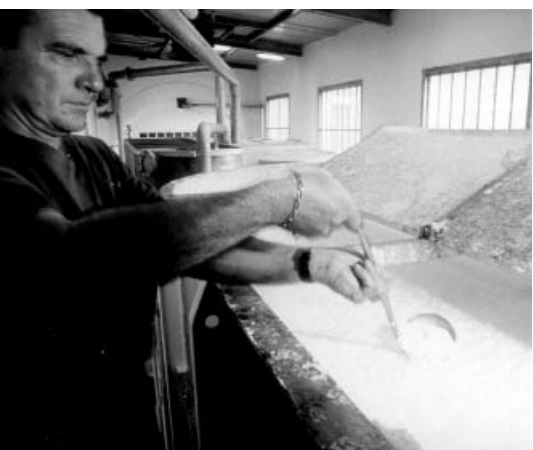
The paper for the euro banknotes is dyed in the mass, each denomination with its own colour.
