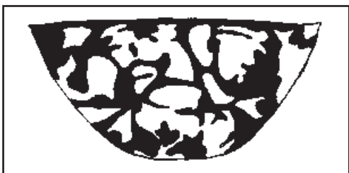
4/ ( Principal step : 85% ) Suspension of solid entities in the liquid; solid size decreases.
