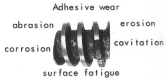
figure 2 : Modes of deterioration in the twin screw extruder
