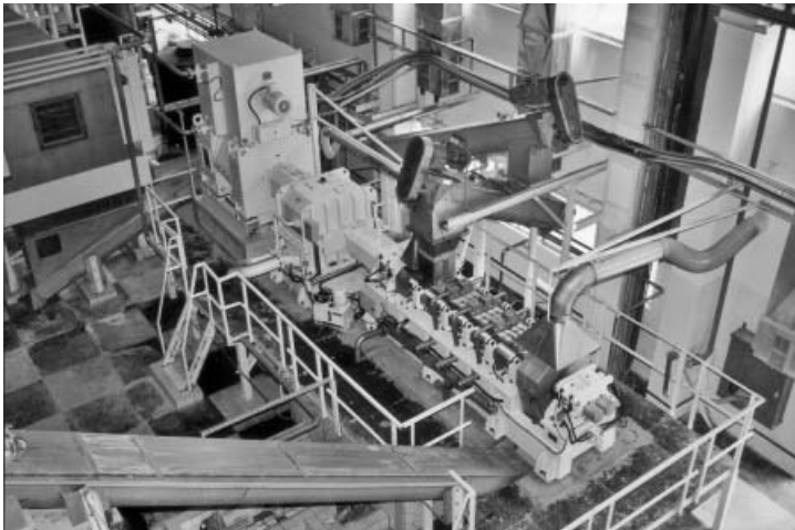
Bivis 2 : fibres cutting, washing and bleaching
