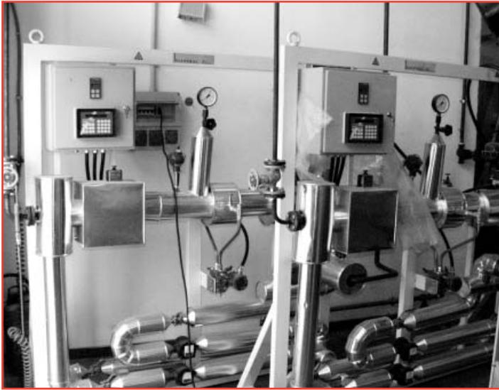
*Steam control units supplying the preconditioner and the extruder.*
