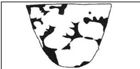
3/ ( Cutting and polishing : 5% ) Deformation of pellets, liquid between pellets; sample density increases.
