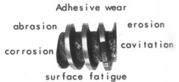
figure 2 : Modes of deterioration in the twin screw extruder
